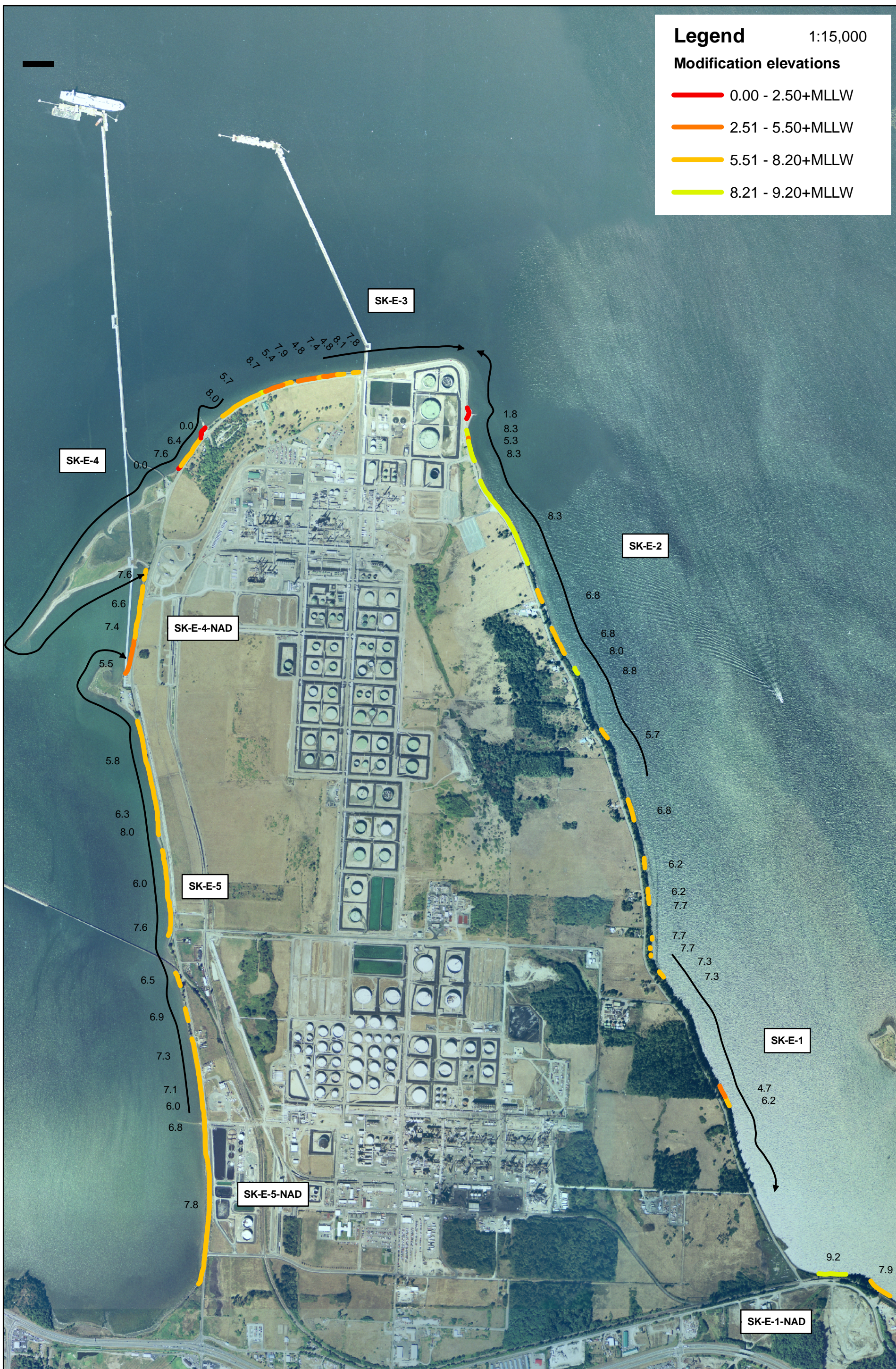
Figure 5. Elevation of all shore modifications along the March's Point shores
