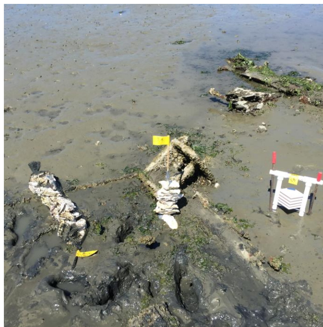
Figure 5. Photograph of post-larval recruitment sampling tools used in Fidalgo Bay. Left: cultch bag of Pacific oyster shells; Middle: shell string (ten shells on a stick - used for PSRF monitoring); Right: ceramic tiles, 5 tiles to a rack.
